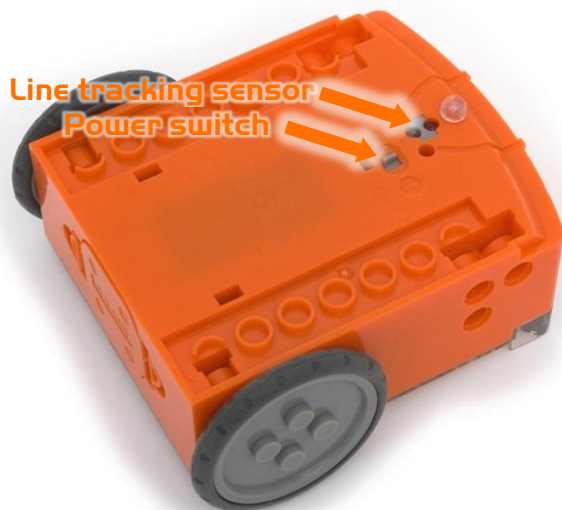
Edison's power switch and line tracking sensor
