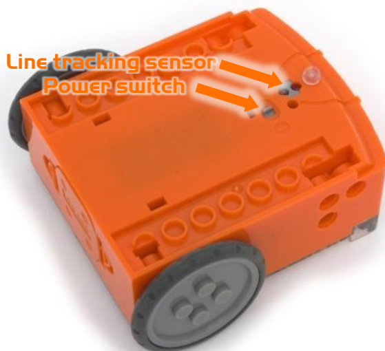
Edison's power switch and line tracking sensor
